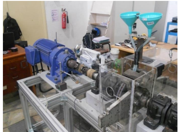
Figure 1: Brake squeal dynamometer test rig
