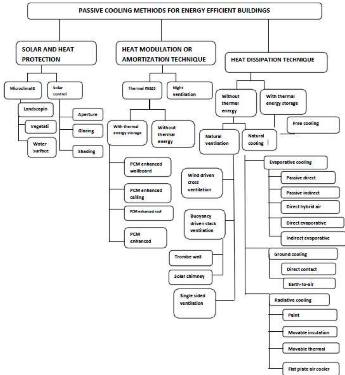
**Figure 2:** Classification of passive cooling methods in energy efficient buildings [2]
