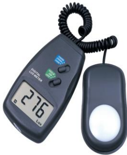
Photo 5: Luxmeter (for the measurement of lighting) (Lx-1010B Digital Light Luxmeter)
