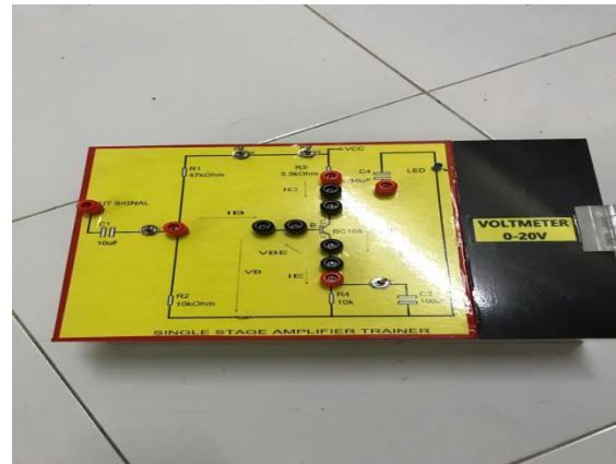
Rajah 2 Single Stage Amplifier with Portable Voltmeter
